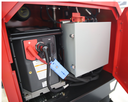
AW16-B: This buggy comes with a compact battery and electronic storage for ease of maintenance.
