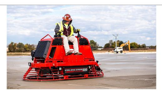
Paragould, Arkansas USA - Allen, a leader in concrete finishing equipment, announced the debut of the 2019 HDX600 Riding Trowel. The new HDX600 is a hydraulically-controlled, eight foot class ride-on power trowel that is powered by a powerful fifty horsepower Hatz liquid-cooled diesel engine.
