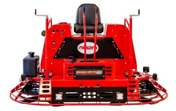
Paragould, Arkansas USA - Allen, a leader in concrete finishing equipment, announced the debut of the MSP465 Riding Trowel. The new machine is a mechanically-driven, eight foot class ride-on power trowel that is powered by a powerful fifty-seven horsepower Kubota liquid-cooled gasoline engine.
