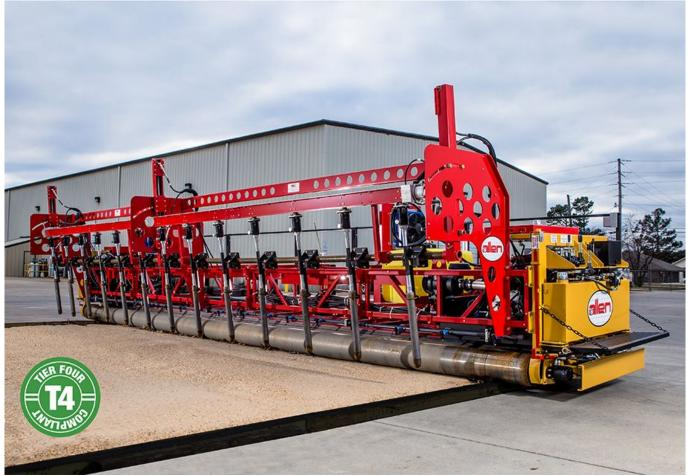
Paragould, Arkansas USA - Allen a leader in professional quality site prep and concrete placing and finishing equipment, announced the debut of their newest form riding paver. The 255T4 is a high production, triple roller tube paver that is great for concrete streets, parking lots, shoulders, ramps, approaches, airfields and more.
