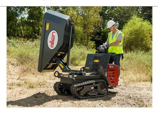
Paragould, Arkansas USA - Allen a leader in professional quality site prep and concrete finishing equipment, announced the debut of their newest track buggy. The AT14S is a swivel dump buggy that allows operator to place materials with precision.
