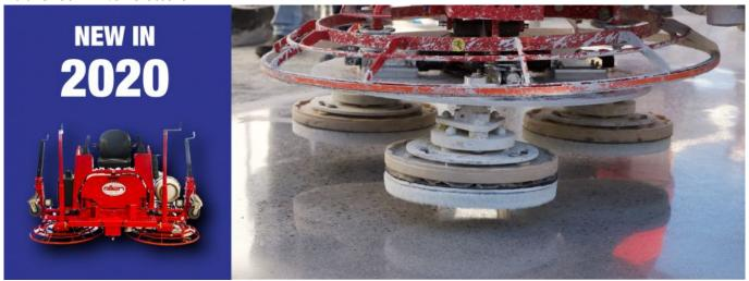
New from Allen Engineering in 2020 - the RP 235 and RP 245 Rider Polishers designed with the high-volume concrete polisher in mind. These riding trowels turned concrete polishers can achieve the necessary high rotor speeds and torque for polishing demanding concrete floors.
