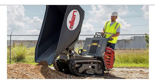
The AT14F rubber track buggy is great for contractors because it is a durable, full-size track buggy that will fit through any standard doorway. This compact machine is equipped with a reliable 20hp Honda engine, easy-to-clean 14 cu. ft. capacity poly bucket, and it is easy to maintain. It is a perfect fit for concrete workers, landscapers, contractors or anyone else who needs to haul or dump material on a regular basis.
