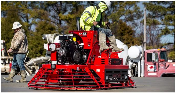
The HP205 riding trowel, features twin Kohler EFI gasoline engines. This Allen rider is a workhorse built for concrete professionals to deliver maximum horse power to the rotors through electronic fuel injection. Utilizing specially tuned torque converter clutches, the HP205 provides excellent low end torque for low speed float panning and superior high rotor speed for burnishing concrete.
