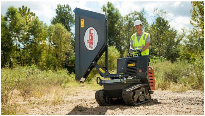
The all new Allen AT14S rubber track concrete buggy delivers excellent performance and precise maneuverability. Equipped with a 90-degree dump angle and 180-degree pivoting dump this buggy can place your material exactly where you need it.
