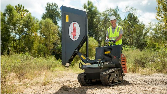
The all new Allen AT14S rubber track concrete buggy delivers excellent performance and precise maneuverability. Equipped with a 90-degree dump angle and 180-degree pivoting dump this buggy can place your material exactly where you need it.
