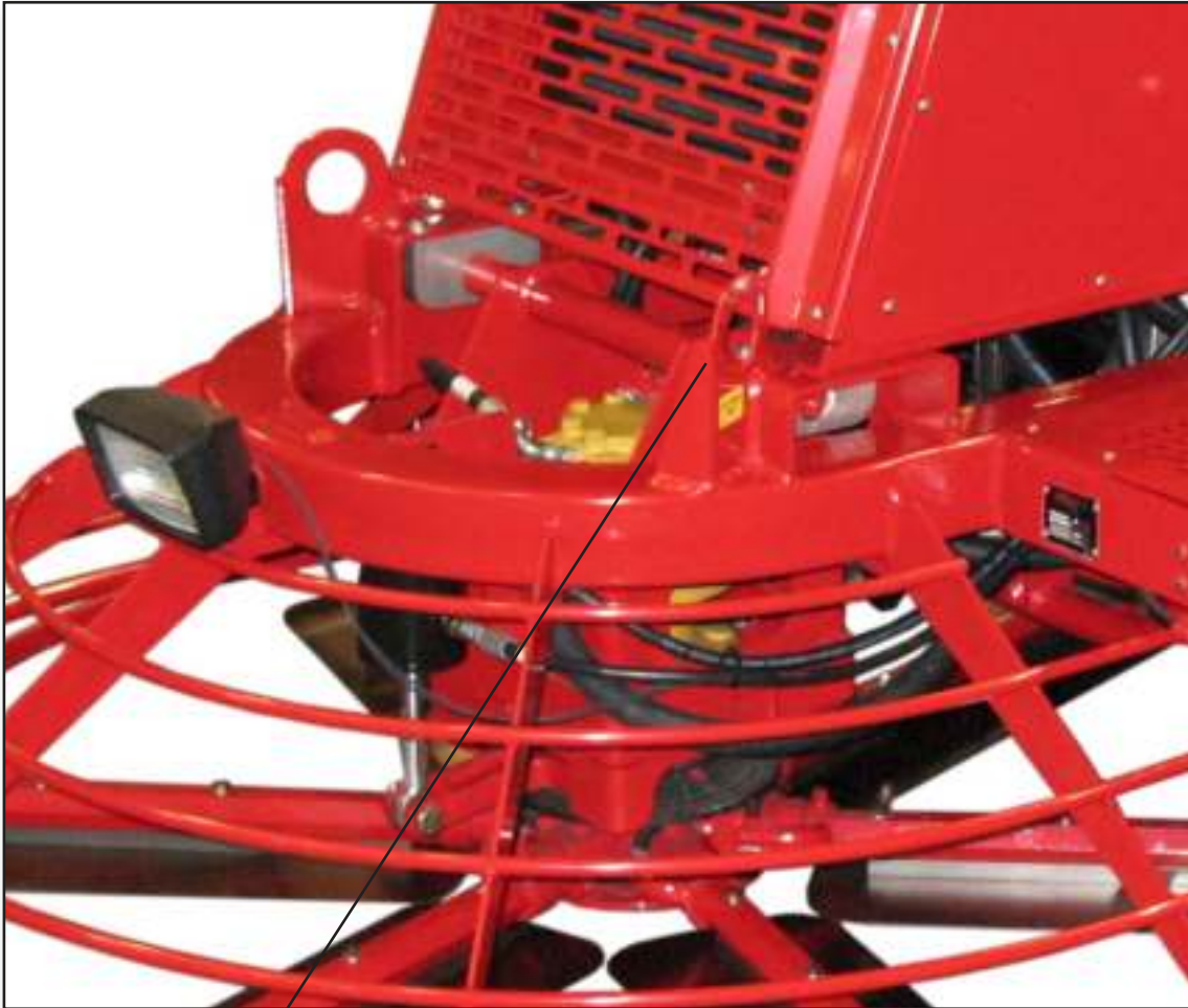
[O] FIGURE 3.4.4 LIFTING HOOK LOCATION
