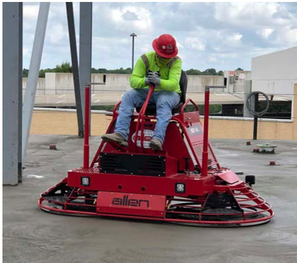
MSP475: Powerful 57 hp liquid-cooled gasoline Kubota engine provides great power for all contractor's finishing needs.
