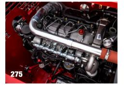
HATZ DIESEL ENGINE Hatz Turbo Diesel 4 cylinder engine boasts 74 HP and offers low fuel consumption. Hatz 74HP is on the 275.
