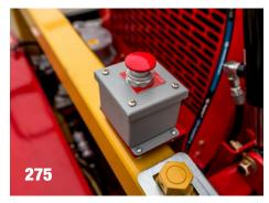
**EMERGENCY STOP** Maximum safety with five Emergency Stop Push Button Switches, plus Horn and Strobe. Standard on the 275.
