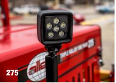
**LIGHTING SYSTEM** Four 35 Watt LED flood lights with adjustable height mounting. Standard on the 275 only.
