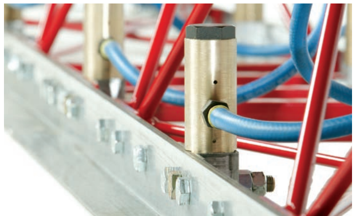
Piston vibrators on 30" centers provide 11,000 VPM to ensure maximum concrete consolidation up to 12" deep.
