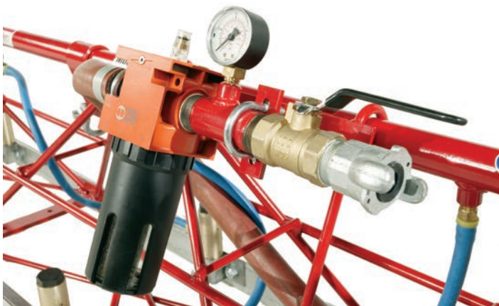
The air flow assembly controls the amount of air going to the machine, and the lubricator ensures proper piston lubrication.
