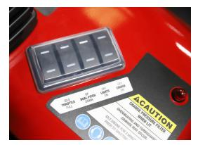
These conveniently located electronic control switches are water resistant.
