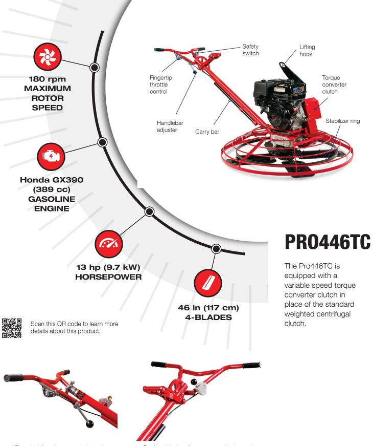
Fine pitch handles use a twist action to control blade pitch from flat to 28° and anything in between.
