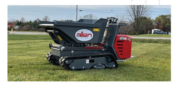
track buggy. Designed for professional contractors, this reliable equipment boasts precise maneuvering capabilities and topnotch performance. The sturdy steel bucket with a 90-degree dump angle and 180-degree pivoting dump ensures accurate material placement, allowing you to achieve superior results every time.
