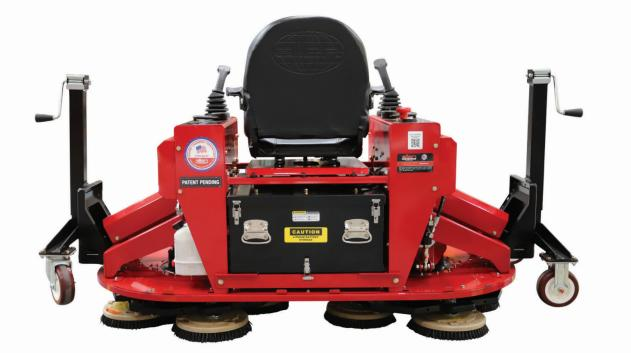
**ROP150-B:** Our innovative design features a conveniently located battery compartment beneath the seat, ensuring effortless access for inspecting and replacing the batteries.
