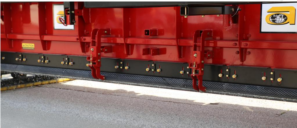
Material is metered through the aggregate bins with the dual auger system and flow is evenly distributed with the helical bar rotation.
