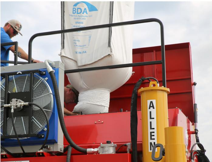
Material loading through the top of material hopper.
