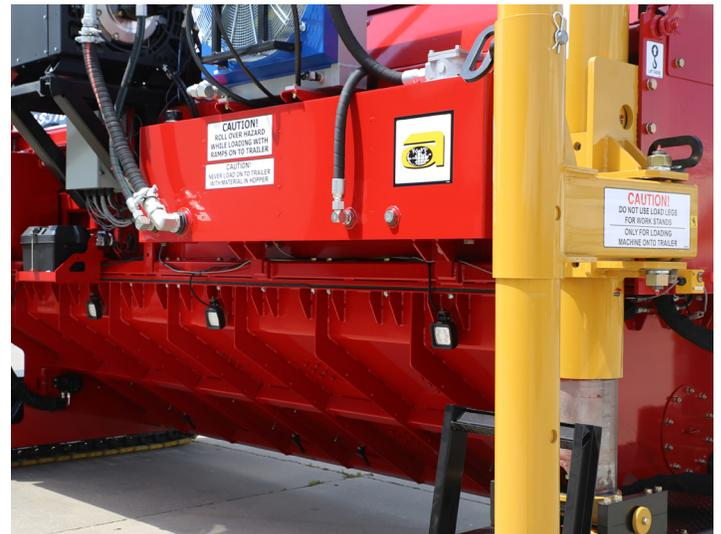
Load leg position extended out from machine prior to loading.
