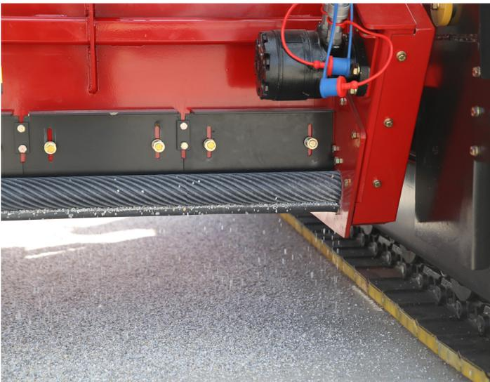
Close up of material distribution through helical bar.
