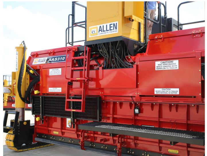
View of the foldable access walkways & ladder to the operator platform.
